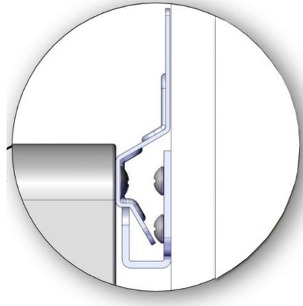
Figure 11: Mount the top bracket
