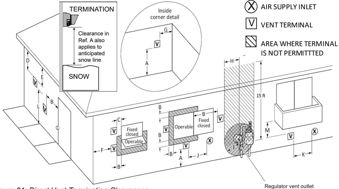
Figure 21: Direct Vent Termination Clearances
