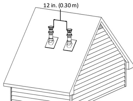
Figure 25: Between terminals at same level
