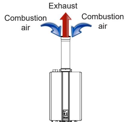
Figure 23: Concentric Pipe
