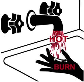
Water temperatures over 125°F (52°C) can cause severe burns or scalding resulting in death.
