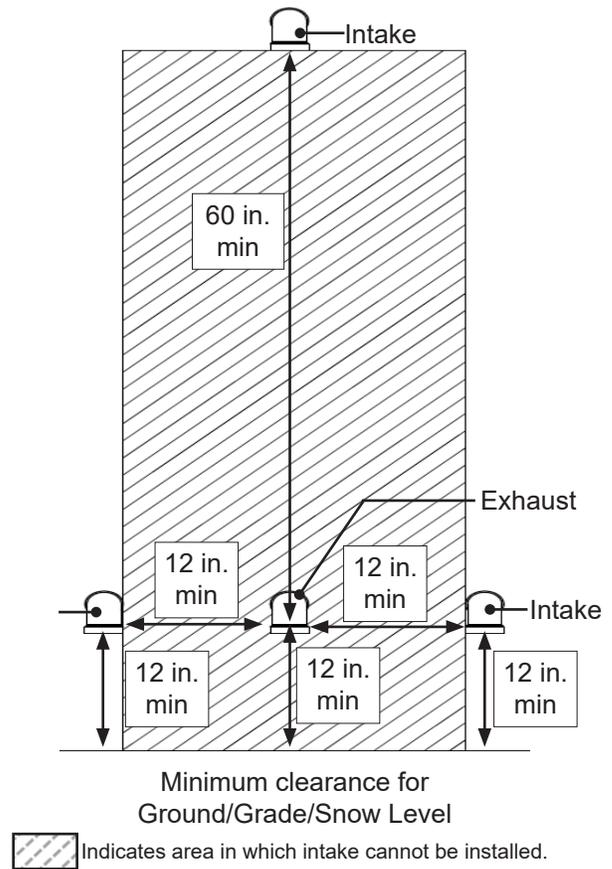
Figure 33: Horizontal Vent and Combustion Air Piping
