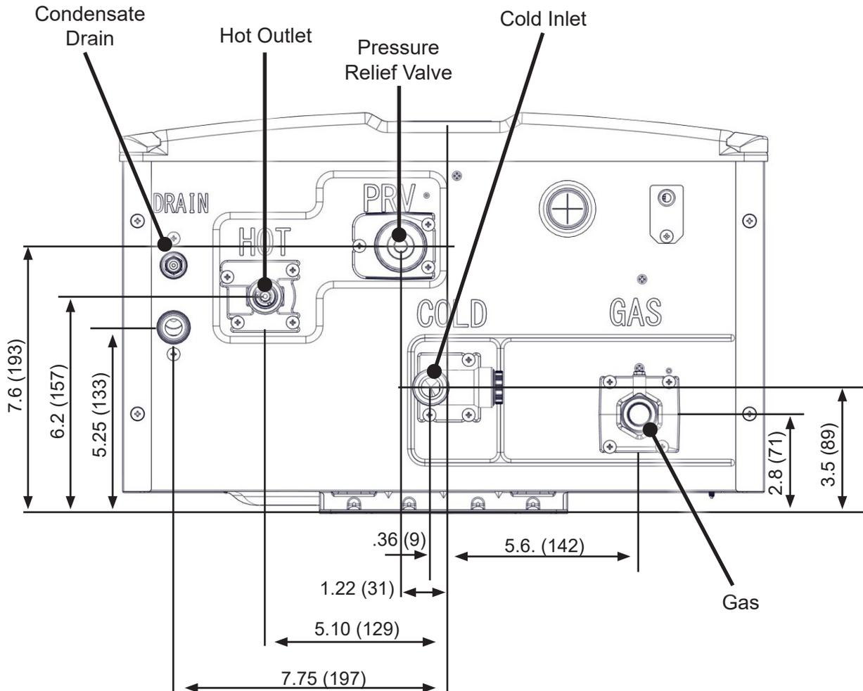
Figure 6: Supply Connections
